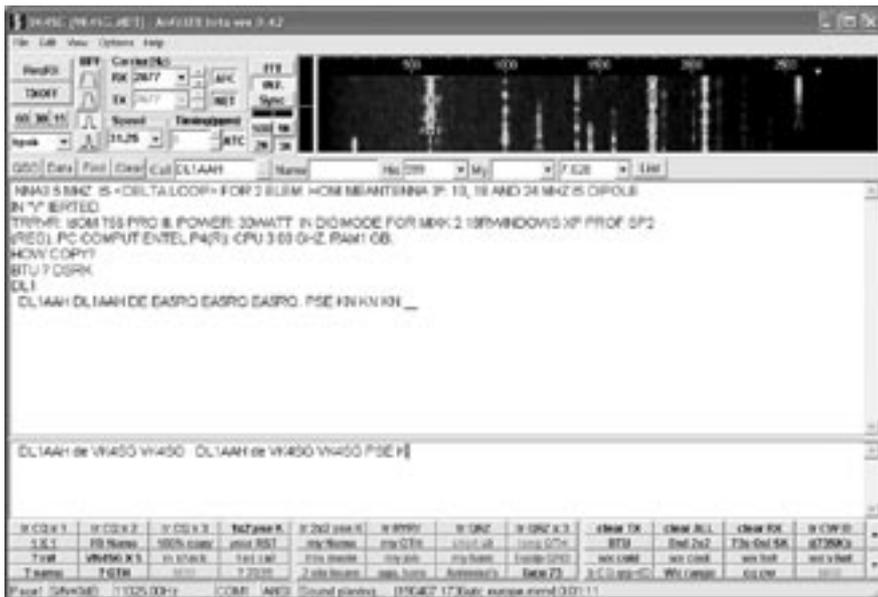
Figure 3: PSK31 signals on 14.070 MHz.
